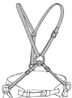
**Upper harness** (shoulder straps and load carrying assembly) are non-PPE elements and not intended for fall arrest
