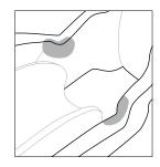
• Check the edges of the attachment hole for wear caused by connectors.
