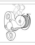
• Check the condition of the swivel (cracks, deformation...).
